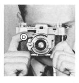
pressing the lever, hold the breath for the instant. If the Kodak is moved during the exposure, the picture will be blurred. *Hold the Kodak steady*.
