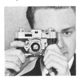
The lens on the Kodak is marked for focusing on the following distances: 4, 5, 6, 8, 10, 15, 25, 50 feet, and INF. (infinity). It is unnecessary to consult this scale when using the range finder, for when the subject is properly focused
